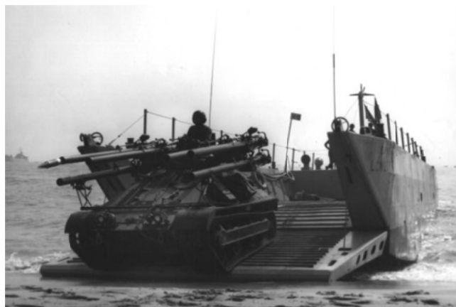
An Ontos hitting the beach Ontos were powered by two Chrysler V-8 engines and were equipped with six 106mm Recoilless Rifles
